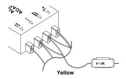
This connection provides power for the CD changer and its components, and continuous power for the CD changer's memory when the ignition is turned off.
